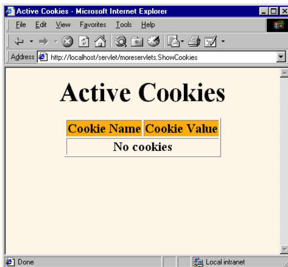
Figure 2-16 Result of visiting the ShowCookies servlet more than an hour after visiting SetCookies (different browser session).
